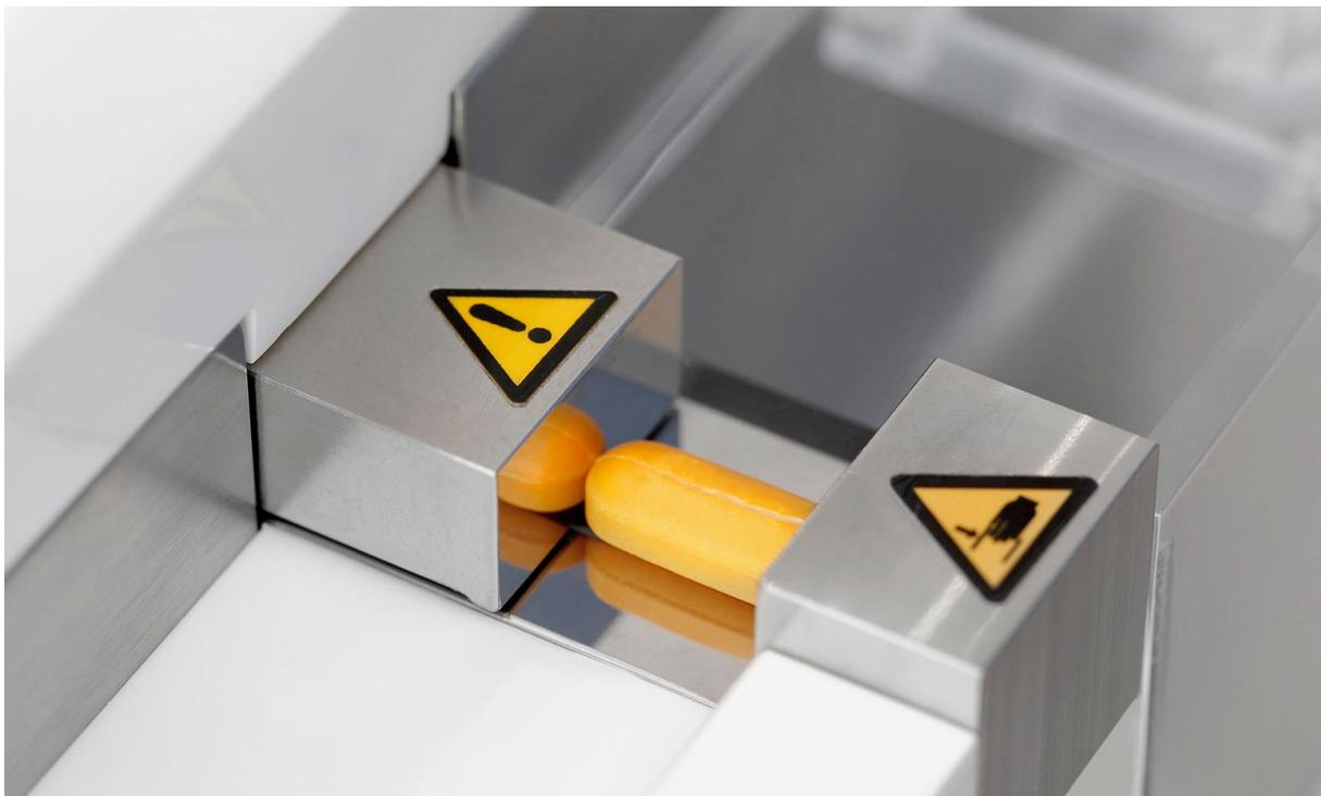
[Charles Ischi AG – Testing Technology](#) is offering fully compliant testing equipment meeting with the revised United States Pharmacopoeia USP-1217 tablet breaking force standards with its automatic QC and [IPC tablet testing system UTS4.1](#) and its [licensed operation Software](#).
